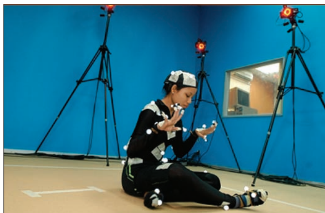
A Mak Yong dancer with motion sensors attached for recording movements during the dance. (Courtesy Info Com Development Centre of Universiti Putra Malaysia.)
