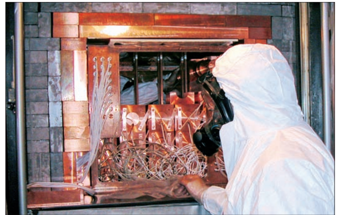
Installing the DAMA-LIBRA detectors in high-purity nitrogen atmosphere.
